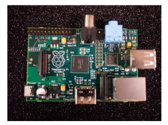
Cryptocat mini-servers will use the Raspberry Pi (<u>http://raspberrypi.org</u>) open hardware for its affordable cost, small size and impressive hardware capabilities.
